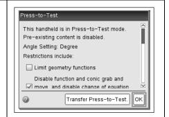
6. During or after the exam, you can tell if a calculator is still in Press-to-Test mode by the flashing LED and also by turning the calculator OFF and back ON. You will again see a confirmation screen.
